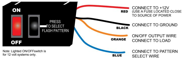
THE PATTERN SELECTION SWITCH IS A MOMENTARY PUSH-BUTTON WHICH SUPPLIES +12V TO BLUE WIRE WHEN PRESSED.
